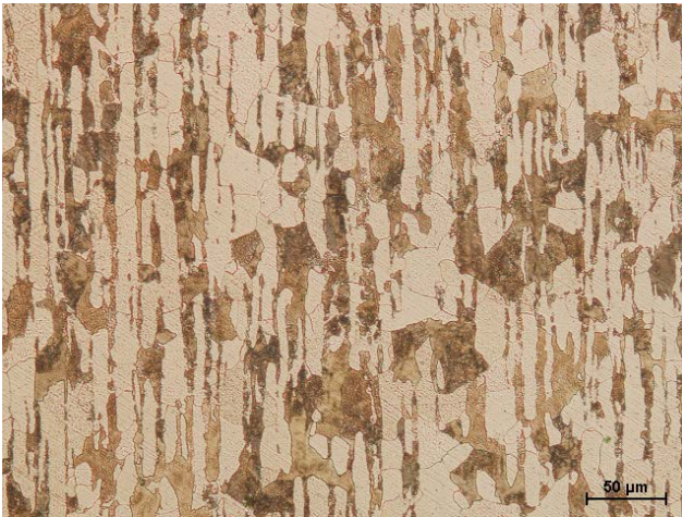
Fig. 3. Ferritic-pearlitic microstructure of the specimen made of 30MnB4 steel cooled with the rate of 0.1°C/s
