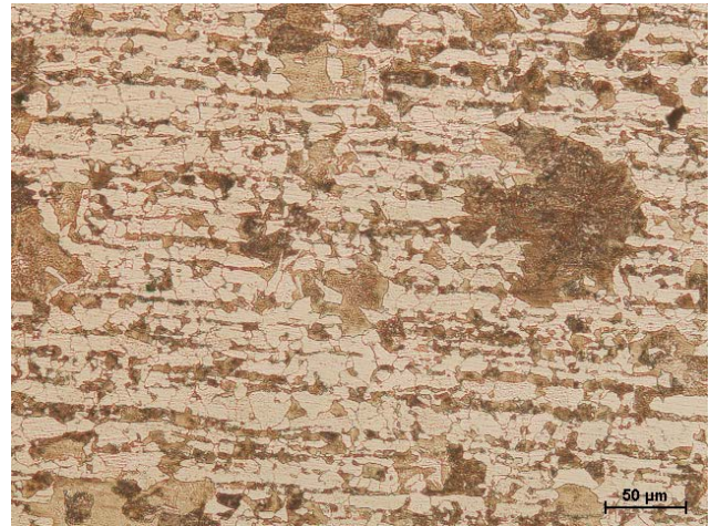
Fig. 4. Ferritic-pearlitic microstructure of the specimen made of 30MnB4 steel cooled with the rate of 1°C/s
