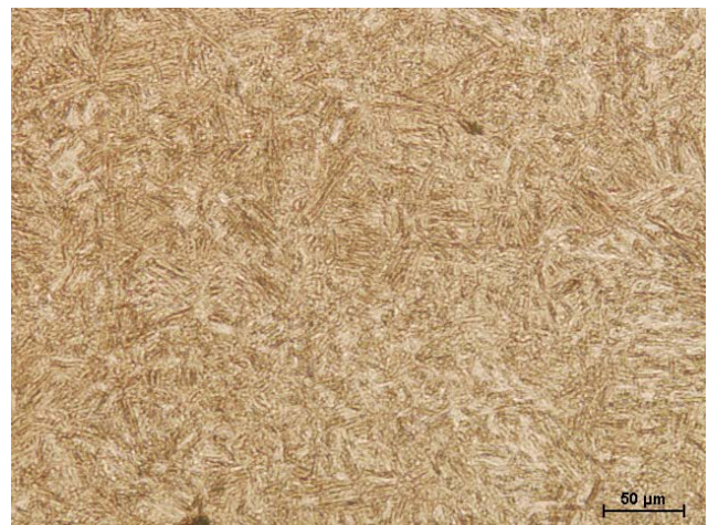
Fig. 8. Martensitic microstructure of the specimen made of 30MnB4 steel cooled with the rate of 100°C/s
