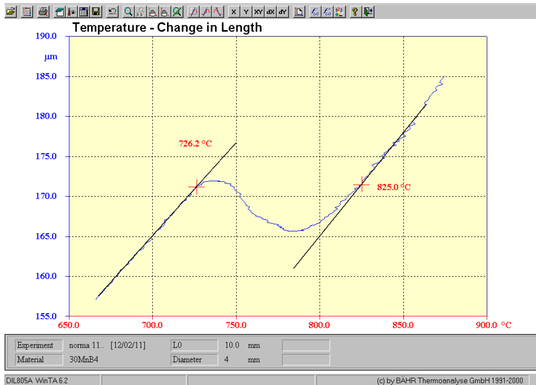
Fig. 2. A dilatometric curve of 30MnB4 steel registered during dilatometric tests and typical temperatures
