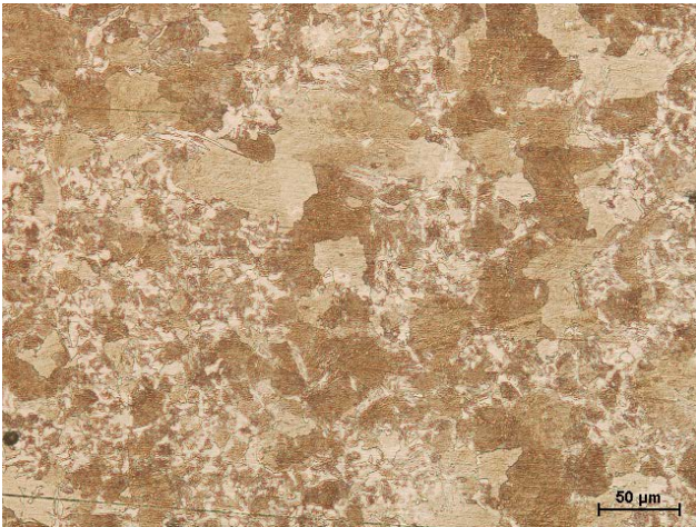
Fig. 5. Ferritic-pearlitic microstructure of the specimen made of 30MnB4 steel cooled with the rate of 5°C/s
